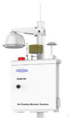
Figure 2: Ambient Air Quality Monitoring Equipment (OCENASUS: AQM-09)
