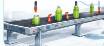
Photoelectric Sensor (Detects defective products)
