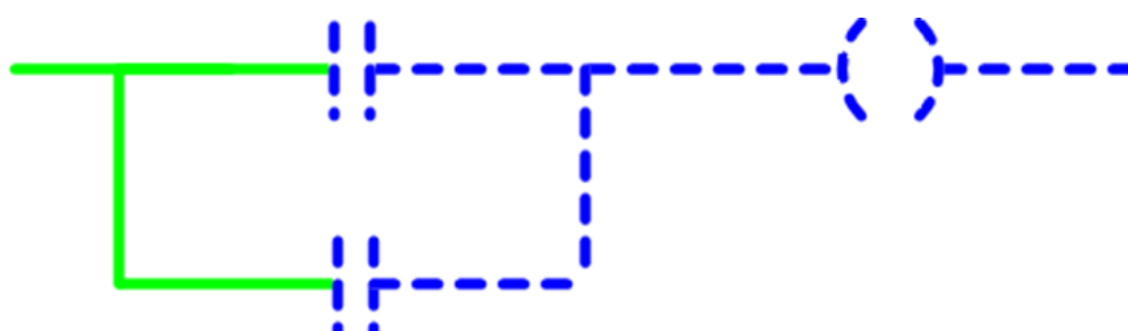
Figure 2.24: AND and OR logic circuits
