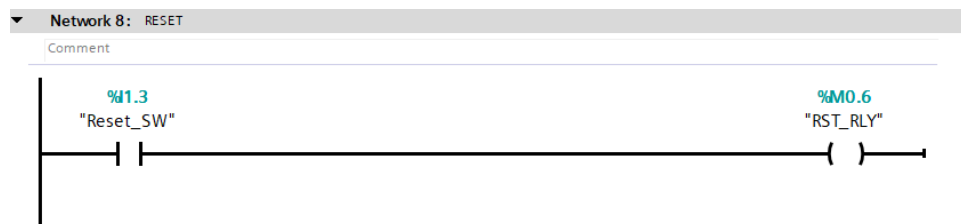
Figure 4.83: Distributing/Conveyor Station Ladder Network 8
