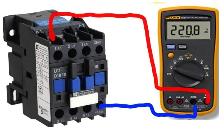
Figure 1.9: Testing relay contacts using a multimeter
